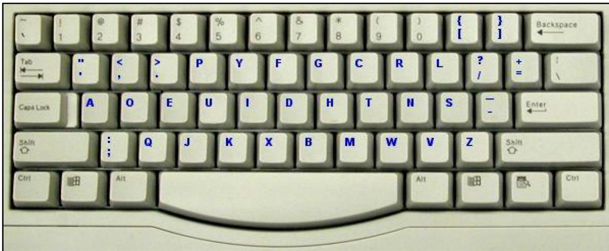
*Fig. 6.6: the make-up of Dvorak keyboard*
