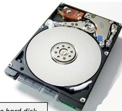
Fig. 6.1: inside the hard disk
